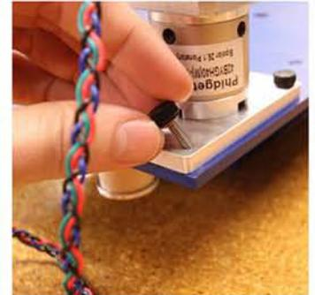
**Step 3:** Attach the pulley to the motor on the underside of the cart.
